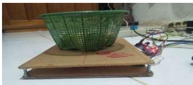
Figure 10. Testing the load cell sensor
