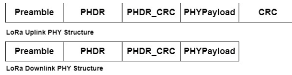
Figure 3. LoRa Uplink and Downlink PHY Structure
