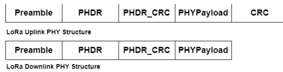
Figure 3. LoRa Uplink and Downlink PHY Structure
